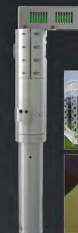
IECHO V-CUT The V-Cut Tool is perfect for producing complex structural designs from foam core or sandwich board materials. The tool can be set for cutting 5 different angles for different cutting requests. The 5 different angles are 0°, 15°, 22.5°, 30°, 45° respectively.
